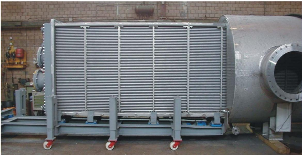
**OELTECHNIK** offers its in-house developed unique bundle trolley allowing for removal and insertion of the bundle on site without additional crane capacities. It assures proper handling of the bundle during maintenance. The bundle cart is adjustable for different shell and bundle sizes so that one trolley can be used for a whole train of EKE Element intercoolers.
