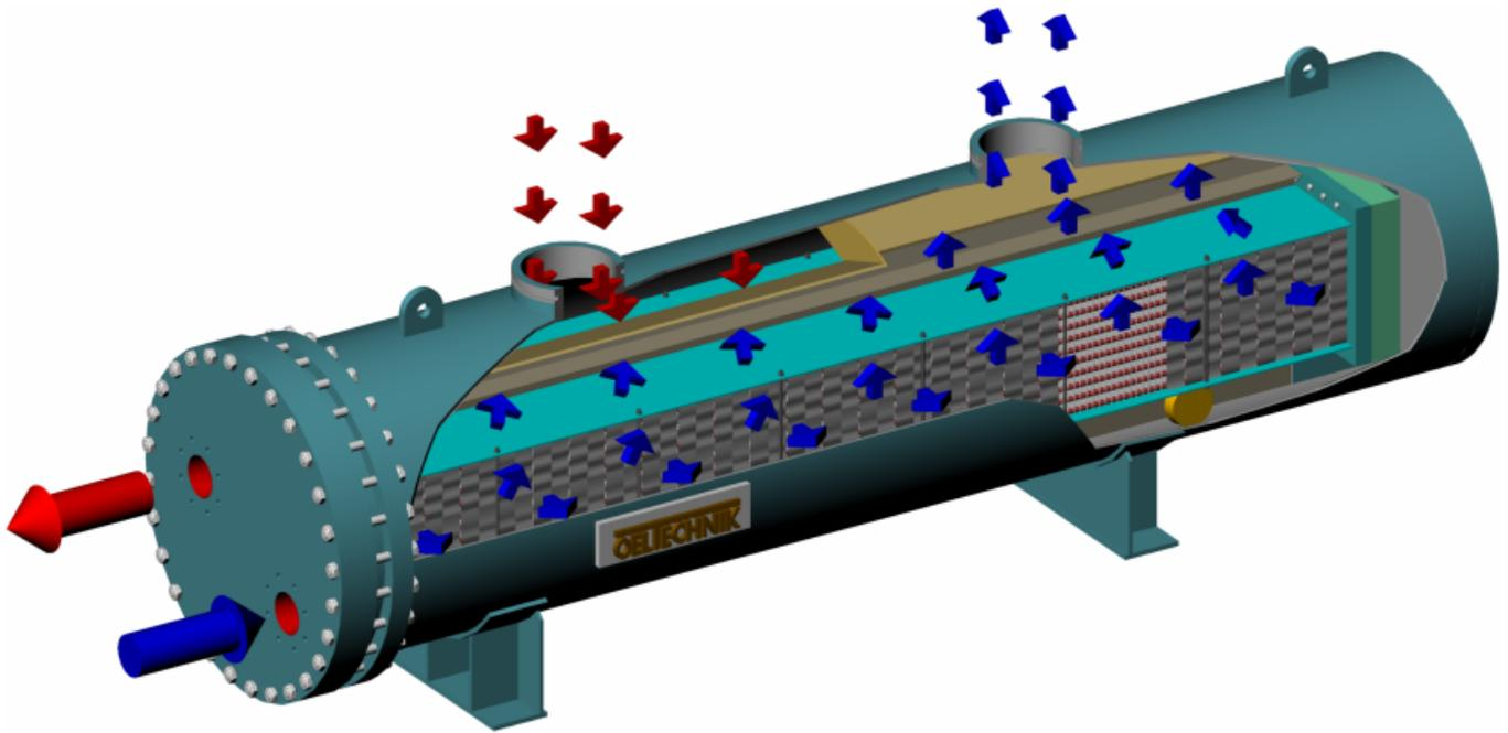
The Type **B3** Element Intercooler is **OELTECHNIK**'s standard bundle form for efficient cooling of wet and dry gases. The gas flow crosses the bundle in one pass. The flow cross sections are optimized by off-setting bundle and shell centerline to achieve the lowest pressure drop possible.
