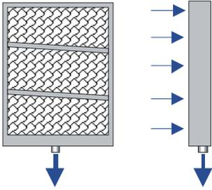
For the B3 Type EKE Intercooler demisters are installed on the gas outlet side of the bundle. A corrosion resistant wire mesh pad is placed in a stainless steel frame. Horizontally inclined gutters ensure the controlled guidance of collected condensate out of the gas stream to the bottom of the shell. From there it is drained out of the intercooler.
