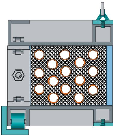
The EKE intercooler bundles show a rigid design. Brass rollers run on stainless steel guides which allow for easy bundle removal and insertion. Stainless steel Y- seals guarantee high performance and long life time. With the three options, plate fin, helical high fin, and Bi-metallic extruded high fin **OELTECHNIK** responds to your individual material requirements.
