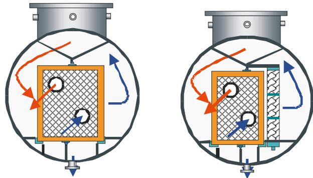
The nozzle locations can be chosen anywhere along the shell only limited by mechanical requirements. For wet gases a vertical demister can be installed to perform internal moisture separation. **OELTECHNIK** has developed and continuously optimized moisture separation devices for years. Separators designed by **OELTECHNIK** allow to cover the specified operating range.
