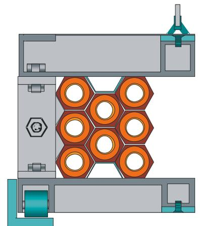
The continuous plate fin enhanced surface interconnects all tubes with each other. The compact packed bundle is fully resistant against vibration. **OELTECHNIK** has developed the plate fin corrugation to maximize the thermal performance of the fins.
