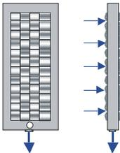
**OELTECHNIK's** wave plate separator is the most space efficient separator design. The waved strips force the gas stream to turn within a small radius. Higher inertial forces let the heavier condensate droplets impinge on the wave plate and drain down, while the gas passes through the waved plate.
