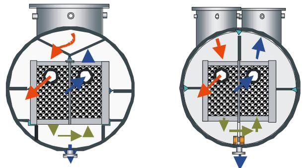
For medium size diameters and high shell diameter to bundle diameter ratios both nozzles can be placed on the centerline. Smaller shell to bundle clearance requires to offset inlet and outlet gas connections.
