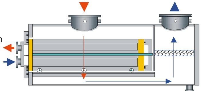
Due to the option to change the bundle location from front to back, an improved adjustment to the compressor design is granted. Nozzles can be inclined to the same side. The design criteria for moisture separation in a vertical flow apply. However the **B1** Type EKE Element Intercooler can be used also for dry gases. A set up turned 90° is also feasible.
