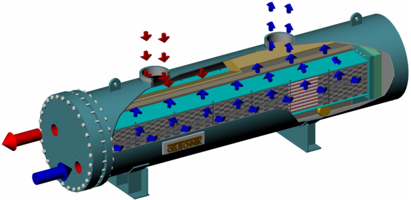
The Type **B2** EKE Intercooler is **OELTECHNIK**'s special design for high efficient cooling of dry gases. A square shaped tube sheet layout is created by an imaginary flipped tube bundle arrangement. This design allows to obtain small vessel diameters. However the advantageous cross- counter flow remains prevailing.
